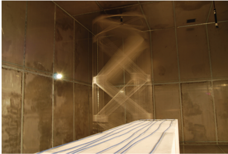
Figure 7: Reverb chamber with rotating vertical tuner and cable under test
